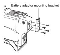
3 Using the wrench and screws supplied with the BKP-L551, mount the BKP-L551 Battery Adapter (not supplied) on the battery adaptor mounting bracket.
